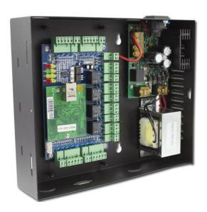
Each AC-170NET units comes in a mountable and lockable metal enclosure integrated with a transfer, power supply/charger, sounder, controller board & backup support for external batteries.
